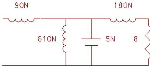
Figure 4. Schematic for single turn transformer model of magnet and beam chamber.
