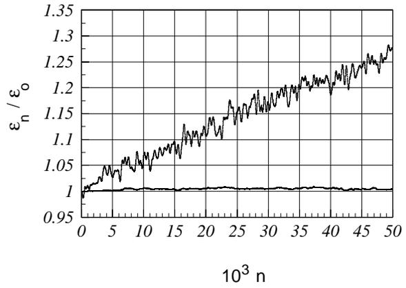
Fig.3. Beam emittance evolution in circular beam-beam interaction with kick (14),  $Q_x = Q_y = 3.175$ ,  $\xi = 0.015$  and 5% noise in  $\sigma$ : (top) without compensation; (bottom) with compensation.
