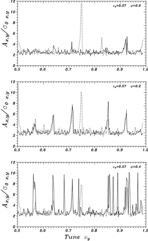
Figure 2: Maximum horizontal ( $A_x/\sigma_x^0$  - solid) and vertical ( $A_y/\sigma_y^0$  - dashed) amplitudes vs.  $\nu_y$ .  $\nu_x = 0.57$ ,  $\xi = 0.025$ ,  $S = 0.6$ , crossing angle  $\phi = 0$  mrad (top),  $0.2$  mrad (center,  $\Phi \simeq 1$ ), and  $0.4$  mrad (bottom).
