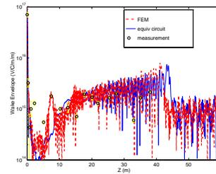
Figure 5: For NLC: Wake envelope comparison between FEM and equivalent circuit method; the circles are measured data.
