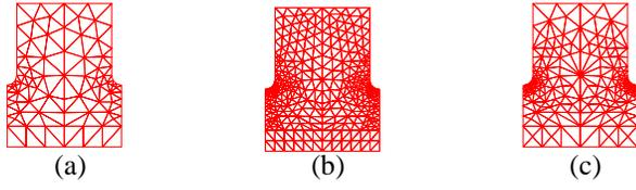
Figure 2: (a) Initial mesh; (b) Uniform refinement; (c) Adaptive refinement.
