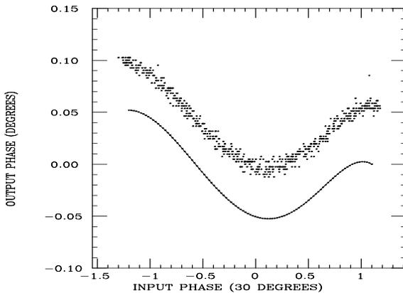
Figure 4: Experimental phase-phase transfer function obtained at the Jefferson Lab injector, and its synthesis using the Tschebyshev expansion (displaced for comparison).
