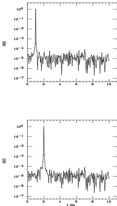
Figure 2: Modulation spectra for  $n = 1$  fundamental and  $n = 2$  second harmonic.
