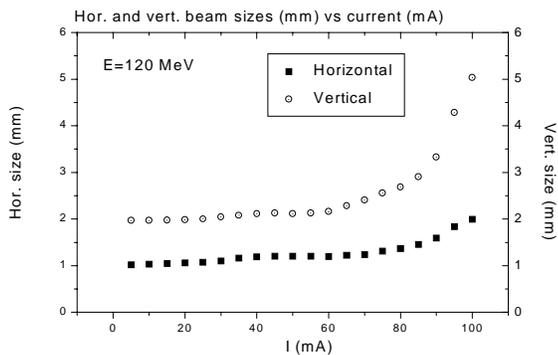
Figure 4a: Horizontal and vertical r.m.s. beam size as a function of beam current for E=120 MeV.
