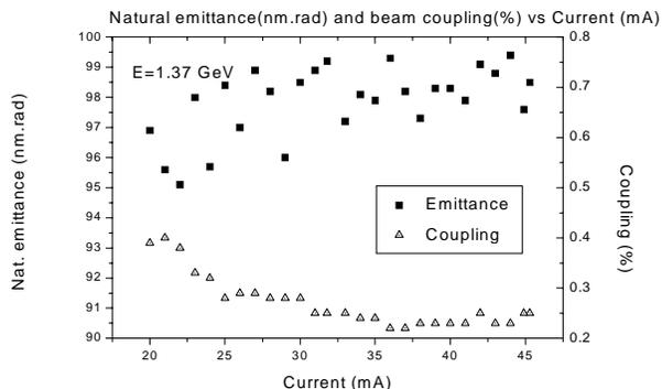
Figure 5b: Natural emittance and coupling as a function of beam current for E=1.37 GeV.
