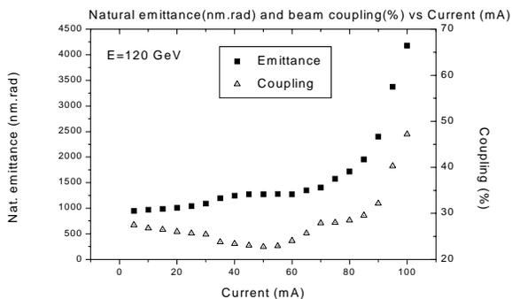
Figure 5a: Natural emittance and coupling as a function of beam current for E=120 MeV.
