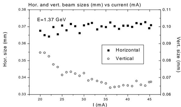
Figure 4b: Horizontal and vertical r.m.s. beam size as a function of beam current for E=1.37 GeV.
