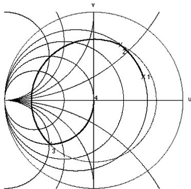
Figure 5: Smith chart representation of double stub matching.
