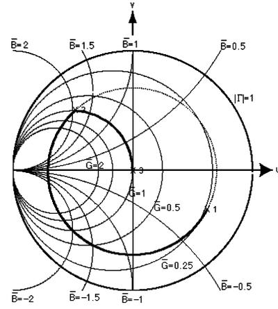
Figure 3: Smith chart representation of the reflection coefficient from a load with mismatched admittance at point 1. A length of waveguide,  $d$ , transforms it on a circle to point 2 where a stub of length  $d_i$  transforms it along a line of constant conductance to a match at 3.
