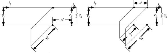
Figure 4: Single (left) and double stub matching(right).
