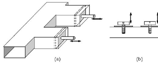
Figure 1: a. Adjustable stub lines perpendicular to the waveguide between the cavity and klystron, b. an equivalent alternative using adjustable posts in the waveguide.
