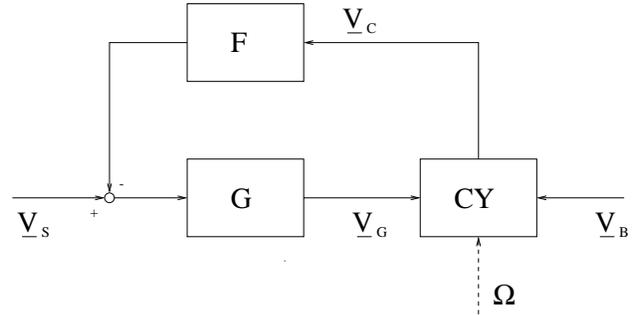
Figure 2: Block diagram of the Petra rf system with G the transmitter gain and F the feedback factor. Voltages  $\underline{V}$  are in complex notation.  $\Omega$  is the detuning value of the cavity CY.
