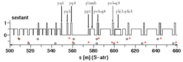
Figure 1: The optical elements in the injection region of the RHIC Yellow ring. Dipole are of height 0.5, quadrupoles are of height 1. The upper (lower) squares show the locations of horizontal (vertical) beam position monitors, the triangles denote orbit correctors. The longitudinal  $s$ -position is taken from the beginning of the transfer line.
