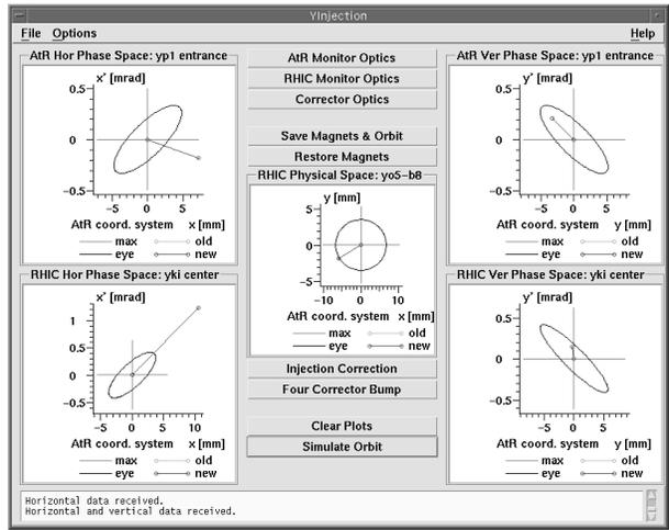
Figure 6: Graphical user interface for the injection tuning program.
