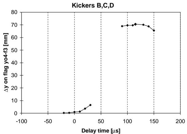
Figure 4: Rise time measurement using only three injection kickers, excluding the “abnormal” one (cf. Fig. 3). The left part of the curve was measured while the corrector yo5-tv9 was powered at its nominal strength; the right part of the curve was measured with 0.25 of its nominal strength.
