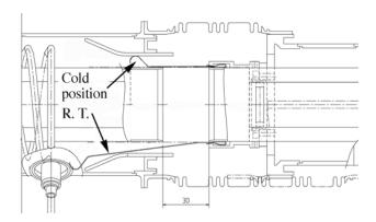
Figure: 5 Beam vacuum interconnection between magnets with a novel RF-bridge design to guarantee flexibility during installation and alignment. Lower section shows room temperature (R.T.) position, upper section shows the contact position at cryogenic temperature.
