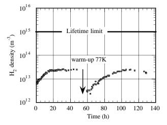
Figure: 4 Evolution of the molecular density of H2 during photon exposure in an experiment at VEPP-2M with a perforated beam screen to simulate LHC during the first running year with 1/10 of the nominal beam current. During the experiment, the screen has been warmed-up to 77 K, while maintaining the cold-bore at ~3K, to the remove cryosorbed hydrogen and thus to demonstrate the repetition of the recycling effect.
