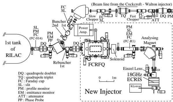
Figure: 1 Schematic drawing of the new injector for the RILAC
