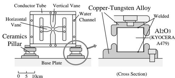
Figure: 3 Schematic drawing of the ceramics pillar.
