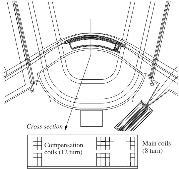
Figure 4: Location of the MIC1 together with its cross section. Injection and the first equilibrium orbits for  $^{16}\text{O}^{8+}$  (200 MeV/u) and  $^{238}\text{U}^{58+}$  (150 MeV/u) are also shown.
