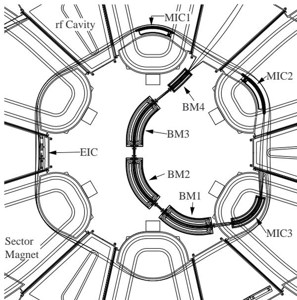
Figure 1: A schematic layout of injection elements for the SRC, and possible trajectories for the injected beam.
