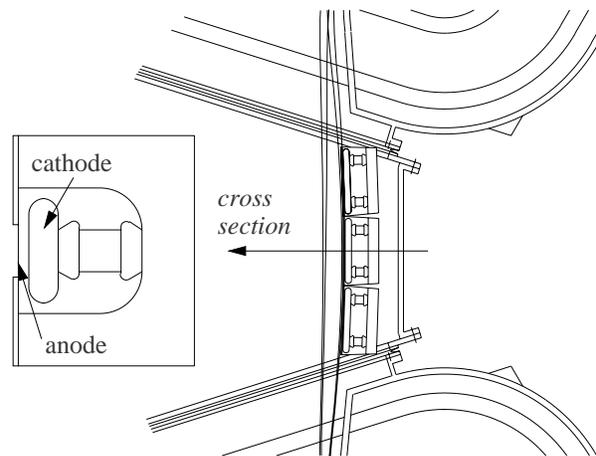
Figure 5: Location of the EIC together with its cross section. The first and the second equilibrium orbits for  $^{16}\text{O}^{8+}$  (200 MeV/u) and  $^{238}\text{U}^{58+}$  (150 MeV/u) are also shown.
