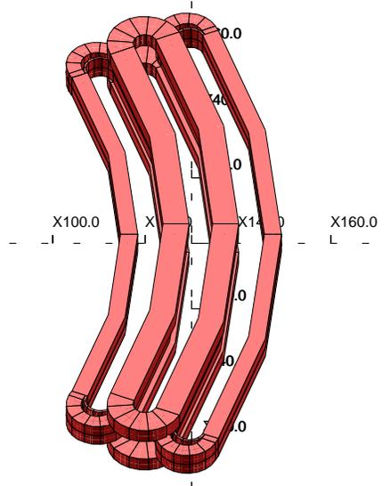
Figure 2: Coil structure of the BM1
