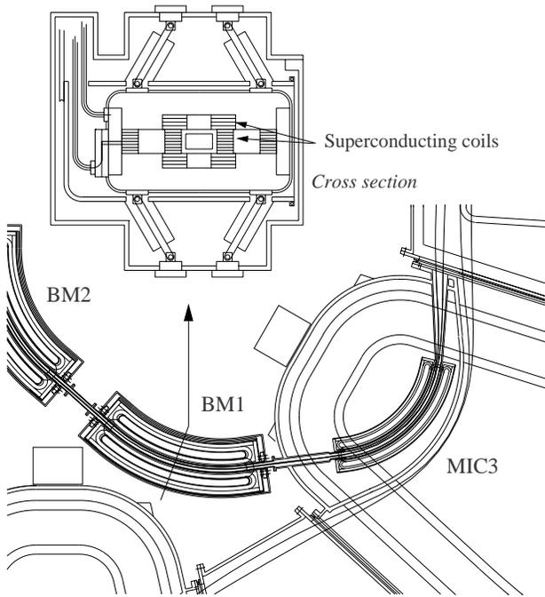
Figure 3: Location of the BM1 in the SRC together with its cross section. Injection and the first equilibrium orbits for  $^{16}\text{O}^{8+}$  (200 MeV/u) and  $^{238}\text{U}^{58+}$  (150 MeV/u) are also shown.
