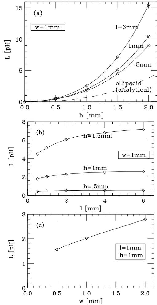
Figure 2: The inductance obtained for a single rectangular post when varying the height  $h$  (a), length  $l$  (b), and width  $w$  (c) (the plotting symbols). The dashed curve in (a) is the analytic result for a half-ellipsoid with radius  $a = .5$  mm[5].
