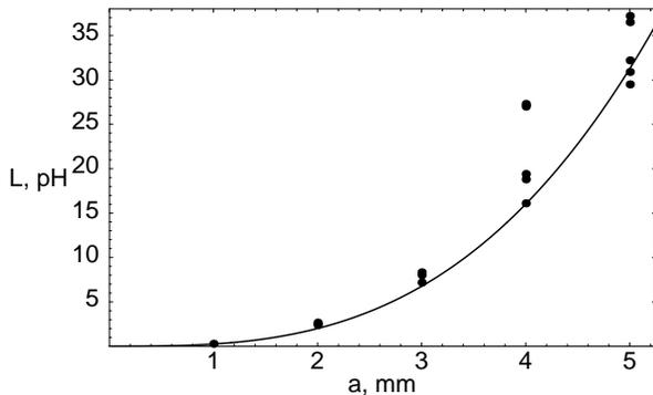
Figure 1: Comparison of MAFIA results (dots) for the inductance of a semispherical protrusion with the analytical ones (solid line) from Eq. (7), for different sphere radii. Pipe radius  $R = 2$  cm.
