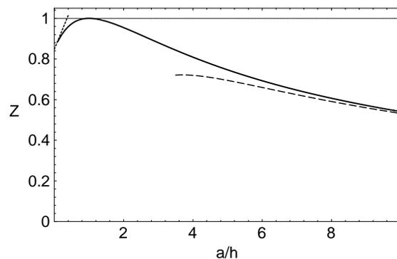
Figure 2: Mask impedance  $Z$  (in units of that for a semisphere with the same depth, Eq. (7) with  $a = h$ ) versus its length. The narrow-mask approximation, Eq. (8), is short-dashed, and the long-mask one, Eq. (9), is long-dashed.
