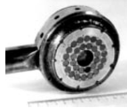
Fig.2. Quadrupole with permanent magnet in a drift tube (the end cover of the tube is removed).
