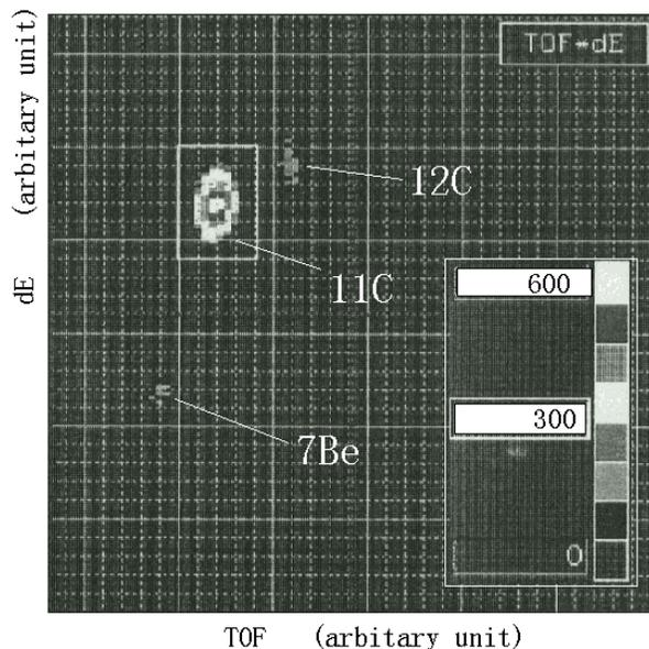
Figure: 4 Scatter plot of TOF vs. delta E obtained in the beam test. Events of  $^{11}\text{C}$ ,  $^{12}\text{C}$  and  $^7\text{Be}$  are clearly separated. The intensity ratio of  $^{11}\text{C}$ ,  $^{12}\text{C}$  and  $^7\text{Be}$  are about 90%, 5% and 5%, respectively.
