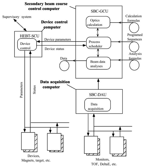
Figure: 3 Block diagram of the control system of the secondary beam course.
