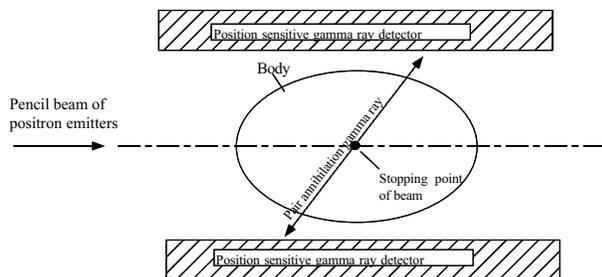
Figure: 5 Method of range evaluation by the positron camera.
