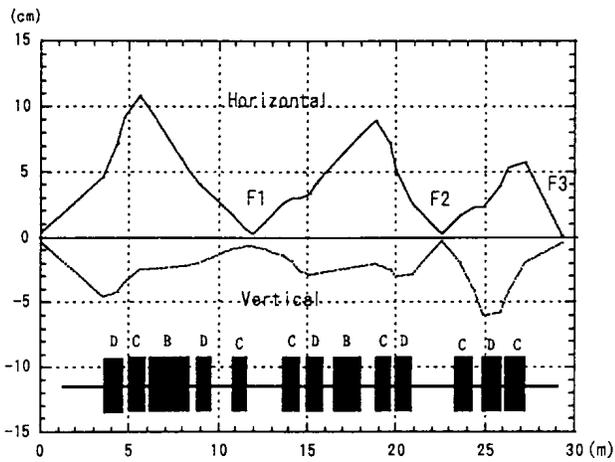
Figure: 2 Beam envelopes of the secondary beam course SB1. Emittance of the vertical and horizontal are assumed to be  $40\pi$  mm mrad at the production target.
