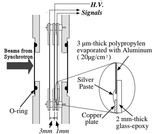
Figure 2: The cross-sectional view of the PPIC. The electrodes are the  $3\mu\text{m}$ -thick aluminized polypropylen film fixed on the 2 mm-thick glass-epoxy frame. Three electrodes can be arranged with front and rear gap distances of 3 mm and 1mm, respectively.
