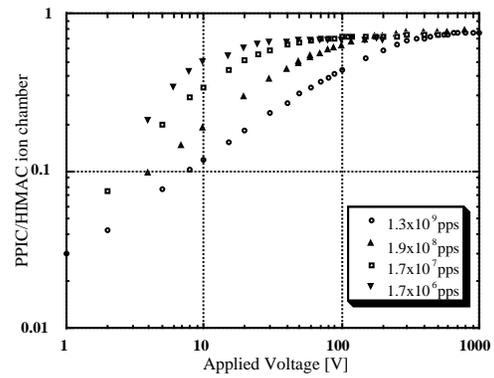
Figure 5: The plateau curve of PPIC(3mm gap distance) with 759.6 Torr air. The beams are  $C^{6+}$  (290 Mev/u). The ordinate is the ratio between the output charge from the PPIC and the HIMAC ion chamber.
