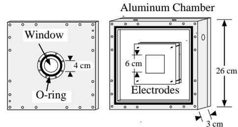
Figure 1: The PPIC. The left figure shows the front lid of the PPIC. The front and rear windows are sealed with O-rings. Three electrodes are mounted in the aluminum chamber.
