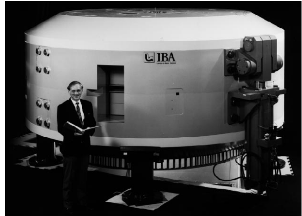
Figure 1: The 235 MeV cyclotron for proton therapy.
