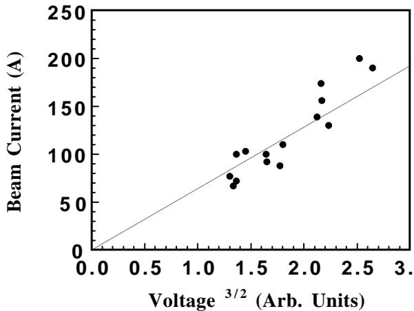
Figure 3: Beam current vs Diode Voltage raised to the three halves power.
