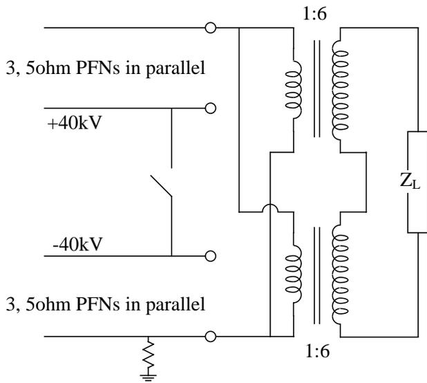
Figure 1: Schematic of pulse transformer.
