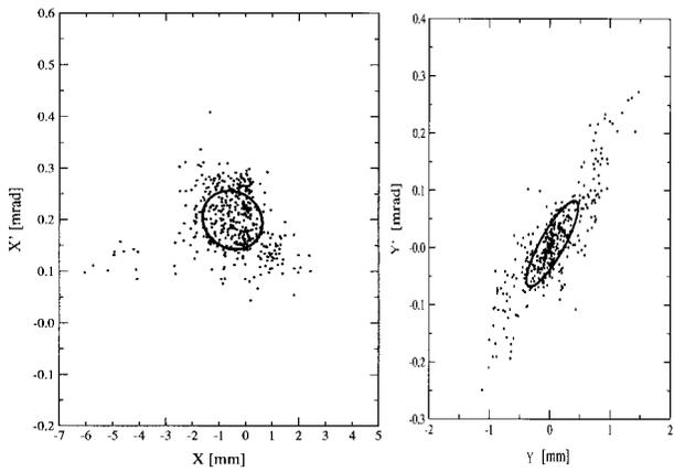
Figure: 4 Calculated  $\epsilon_x$  and  $\epsilon_y$  (rms) of 150 MeV beam.
