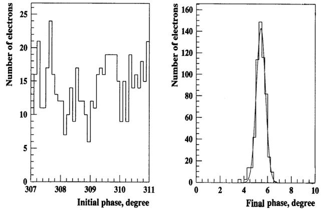
Figure: 7 Effective bunching of RTM from broad initial phase to narrow final phase.
