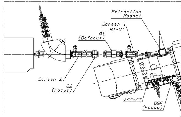
Figure: 2 Device layout used in emittance measurements.
