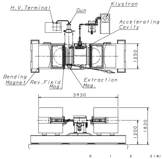
Figure: 1 Top view of 150-MeV microtron with conventional injection system.
