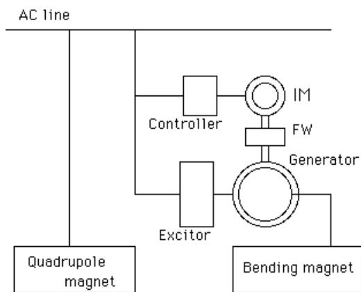
Fig. 6. One idea of a power supply system for the bending magnet
