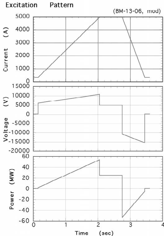
Fig. 5. An example of an excitation pattern of the bending magnet
