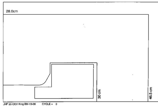
Fig. 1. Cross sectional view of the bending magnet
