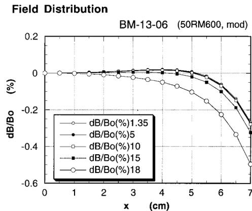
Fig. 2. Field distributions of the bending magnet
