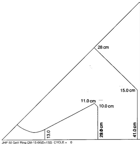
Fig. 3. Cross sectional view of the quadrupole magnet
