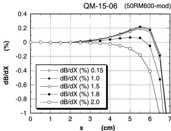
Fig. 4. Distributions of field gradient view of the quadrupole magnet
