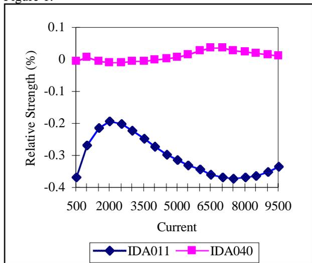
Figure 1. Strength variation vs. excitation for two dipoles, one early and one later in production.
