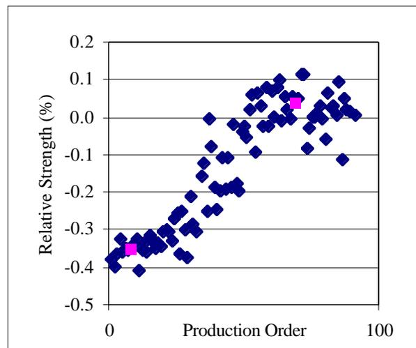
Figure 2. Relative strength at 13.8 kG for the dipoles for the early dipoles, in order of production. The two dipoles shown in Figure 1 are denoted with different symbols.
