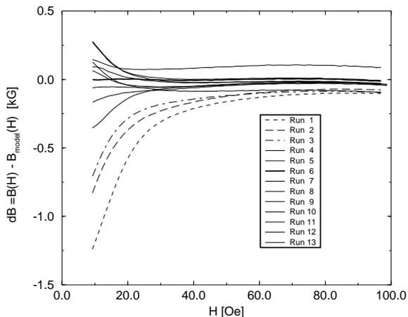
Figure 3.  $B(H)$  curves averages for each of the thirteen runs of steel, relative to a fit to run 6.
