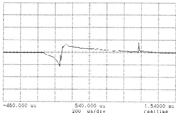
Fig. 3.  $H^-$  beam current on Faraday cup with complete over-cesiation, (1 mA per division) 10 mA present before occurrence of over-cesiation.
