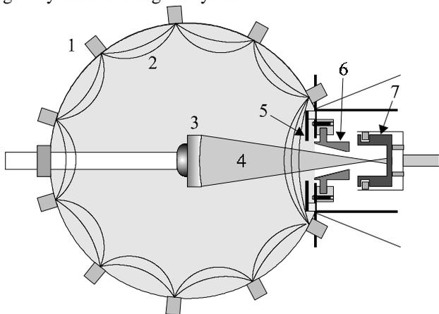
Fig. 2. Schematic of source interior (1. Cusp Magnet, 2. Cusp Field, 3. Converter, 4.  $H^-$  Beam, 5. Aperture Plate, 6. Aperture Cone, 7. Faraday Cup).
