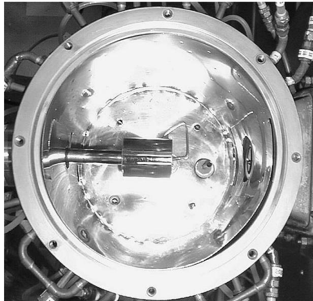
Fig. 1. Close-up of LBNL surface conversion source interior (top down view).
