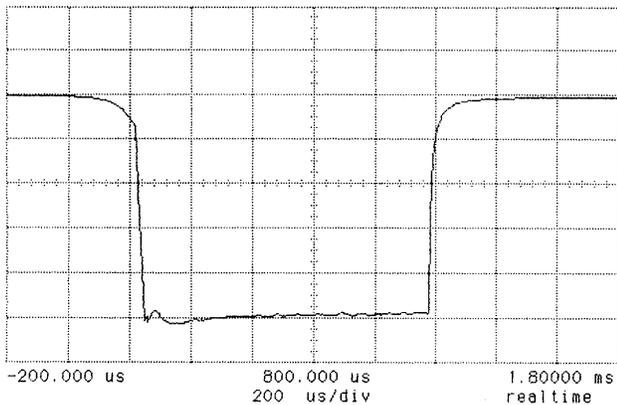
Fig. 4. 20 mA of  $H^-$  beam current on the Faraday cup.
