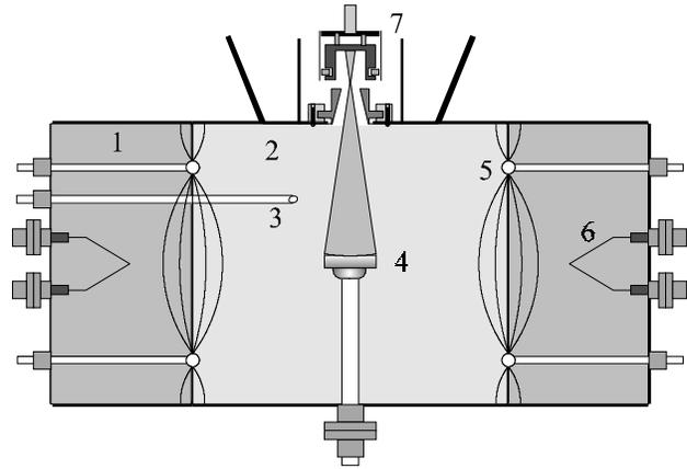
Fig. 5. Source schematic with chamber extensions and magnetic filter (1. High  $T_c$  Region with Filter, 2. Low  $T_c$  region with Filter, 3. Cesium Nozzle, 4. Converter, 5. Magnetic Filter, 6. Filament, 7. Faraday Cup).
