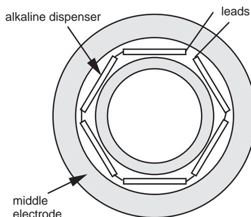
Figure: 3 Front fed vapor source dispenser layout.
