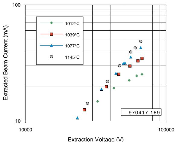
Figure: 6 I-V characteristics for the cesium vapor ionizer.
