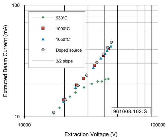
Figure: 4 I-V characteristics for the alumino-silicate K<sup>+</sup> ion source and the doped source.
