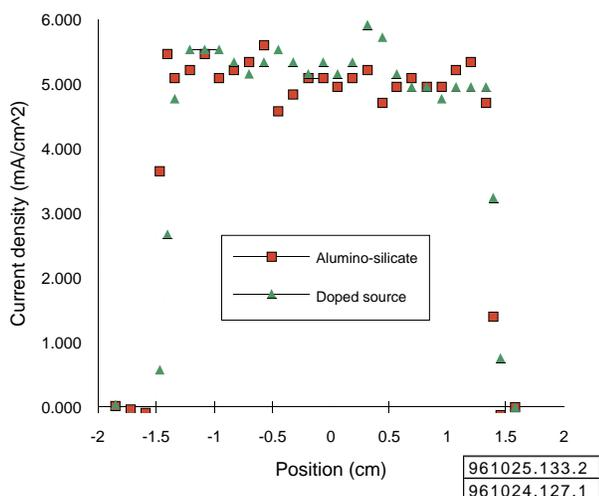
Figure: 5 Beam profiles for the alumino-silicate ion source and the doped source.
