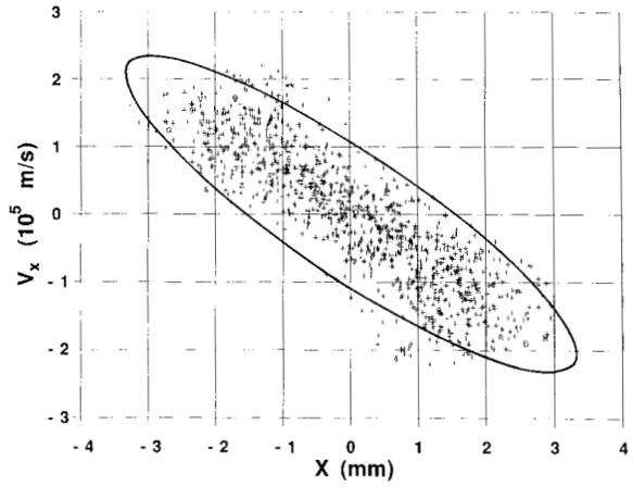
Fig. 3. SCHAR-calculated phase space (crosses) at the RFQ match point for the baseline LEBT design (Case No. 1). The curve is the RFQ acceptance ellipse for a 110-mA,  $0.20\text{-}\pi$  mm mrad beam.
