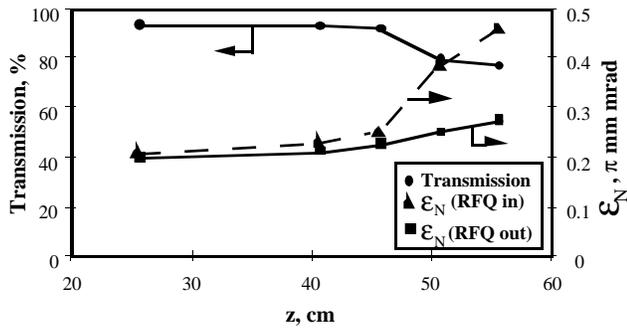
Fig. 5. PARMTEQM-calculated RFQ transmission (circles) and output  $\epsilon_N$  (squares), and SCHAR-calculated RFQ input emittance (triangles) as a function of the distance between Solenoid #2 and the RFQ match point.
