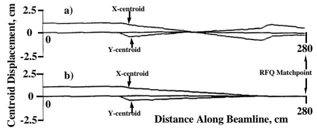
Fig. 6. a) Beam centroid motion for an initial 1 cm offset. b) Beam centroid motion after steering.
