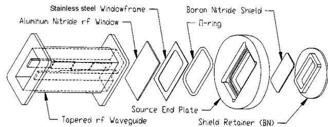
Figure 2. LEDA proton source microwave window.
