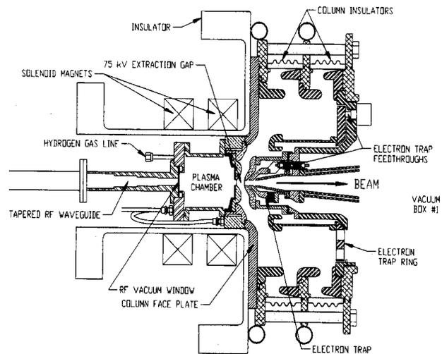
Figure 1. LEDA proton source and HV column.
