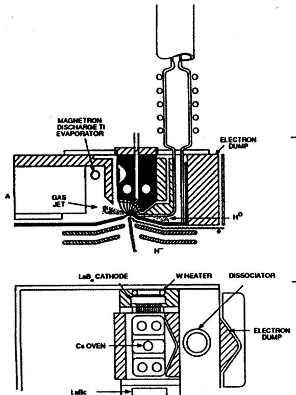
Fig. 2 Basic operating principles and the construction features of the modified SITES SPS.
