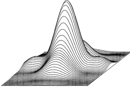
Fig. 6 The PSF at the balanced astigmatism point. The side length of the 3-dimensional plot is 96  $\mu\text{m}$ .
