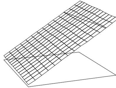
Fig. 3 A result of wavefront by the Shack-Hartmann wavefront sensor. Flatness of the wavefront is less than  $\lambda/20$ . The side length of the 3-dimensional plot is 35 mm.
