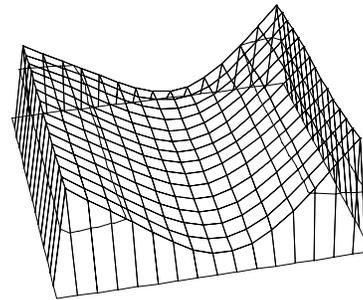
Fig. 5 The surface deformation of the Be-mirror. The side length of the 3-dimensional plot is 35 mm.
