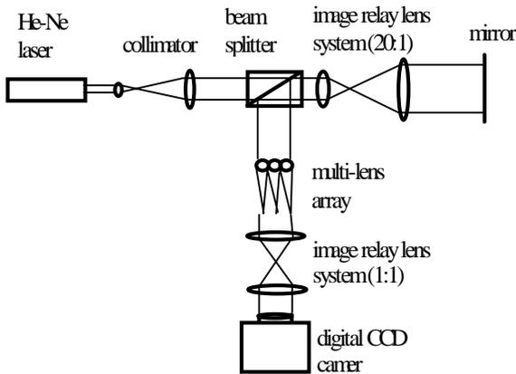
Fig. 2 the system of the Shack-Hartmann wavefront sensor
