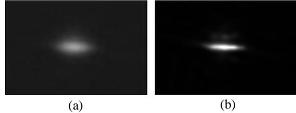
Fig. 7 A beam image of the Photon Factory. The ring energy is 1 GeV and the beam current is 1 mA. (a), The observed image of the beam; (b), the beam image after deconvolution process.
