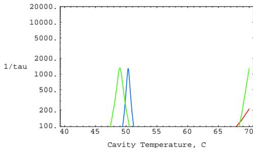
Figure 3: The shifting of horizontal transverse coupled bunch modes with a adjustable HOMFS on cavity S9. 2.0 GeV, 250 mA. Before installing the adjustable frequency shifter (upper graph) and after (lower graph).
