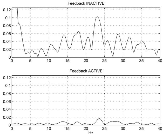
Figure 2. Results of local orbit feedback at ID\_6 in compensating low frequency disturbances.
