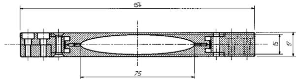
Figure 1: Cross-section of vacuum pump free insertion device chamber.
