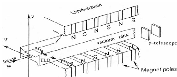
Figure 1: ALS insertion device showing coordinate system, vacuum tank, TLD and  $\gamma$ -telescope
