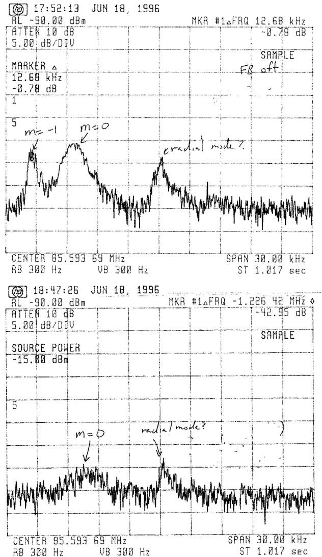
Figure 4: Spectrum of vertical monitor signal just above threshold ( $I=22$  mA.) The left plot is with FB off and right with FB on. The  $m = -1$  mode signal disappears with FB on and the  $m = 0$  signal is depressed. The signal at the zero current vertical betatron tune is not understood but may correspond to a radial mode.
