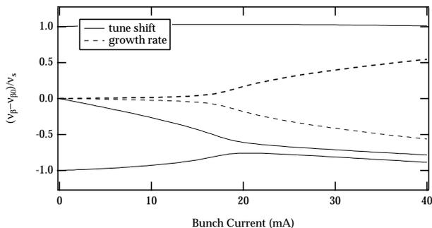
Figure 1: Example calculation of mode coupling instability using the MOSES code. The solid lines show the tune shift of the  $m=0, \pm 1$  modes. The dashed lines show the growth (and damping) rates of the coupled modes above threshold.
