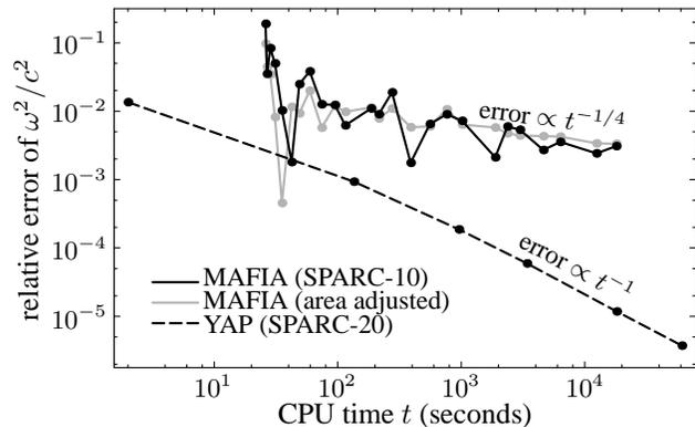
Figure 2: Relative eigenvalue error versus CPU time for MAFIA and the FEA code YAP. The test structure is a pillbox cavity with radius  $\rho = 1$  and height  $l = 1$ . The YAP results are electric field calculations. The MAFIA results employed a uniform grid.
