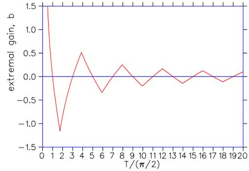
Figure 2: Maximum values of gain,  $b$  compatible with stability versus delay  $T$ .
