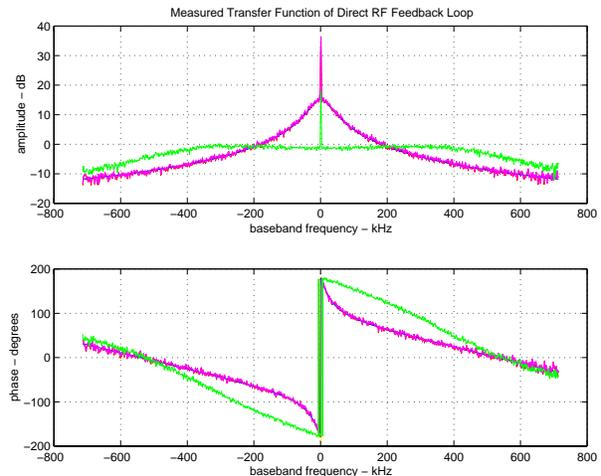
Fig. 3. Measured open/closed loop response of direct loop.
