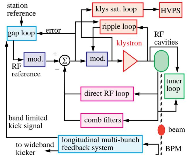
Fig. 2. Block diagram of RF feedback loops used in the PEP-II low-level RF system. Multi-cavities not shown.
