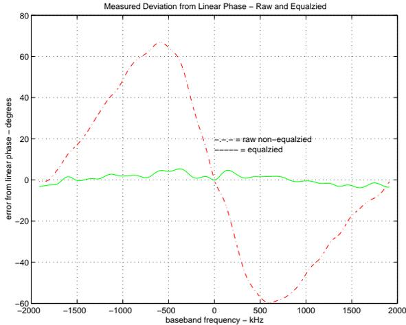
Fig. 4. Measured response without/with equalization.
