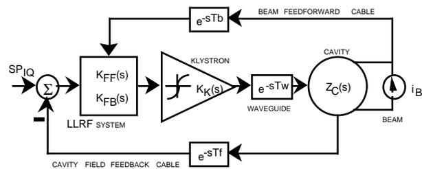
Figure 1. LLRF control system model block diagram.
