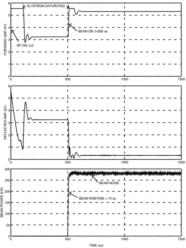
Figure 3. Normal RF and beam turn-on. Forward signal out of klystron, cavity reflected signal, beam power in the cavity.
