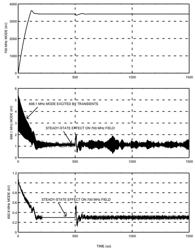
Figure 4. Normal RF and beam turn-on: cavity modes excited.
