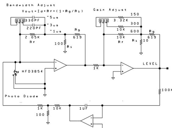
Figure 2. Photodiode Preamp Schematic
