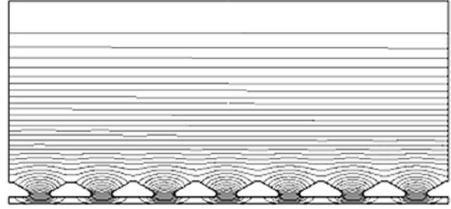
Figure 2: TM<sub>010</sub> Electric field lines in tank #1
