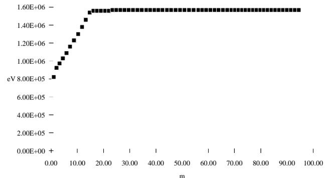
Figure 1: Energy gain per meter vs. MTDTL length.
