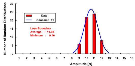
Figure 1: Histogram of Dyn.Aper. (60 seeds) for the nominal LHC lattice including a Gaussian fit
