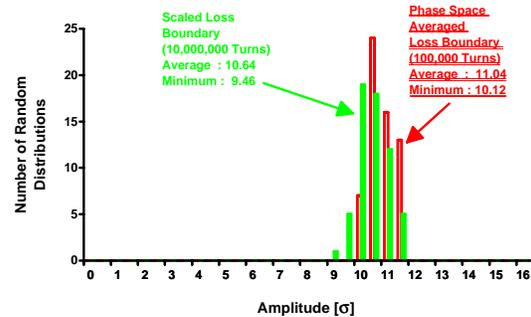
Figure 3: *Scaling of the loss bound histogram from  $10^5$  to  $10^7$  turns*
