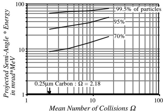
Figure 7: Plural beam scattering of highly relativistic electrons into thin materials. The number of collisions  $\Omega$  is equal to  $0.78 \rho t [(Z+1)Z^{1/3}]/A$  where  $\rho$  is the density in  $\text{g}/\text{cm}^3$ ,  $t$  the beam path length in the material in  $\mu\text{m}$ ,  $Z$  the atomic number, and  $A$  the atomic weight.
