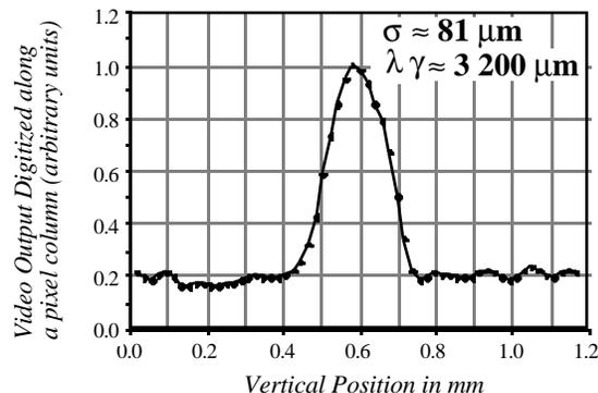
Figure 3: Vertical profile of a 3.245 GeV and 3  $\mu$ A continuous beam.
