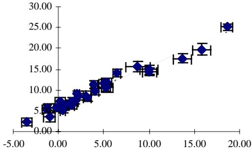
Figure 3: Second moment ( $\text{mm}^2$ ) versus  $\bar{x}^2 - \bar{y}^2$  ( $\text{mm}^2$ ). The slope is equal to  $0.95 \pm 0.03$ .
