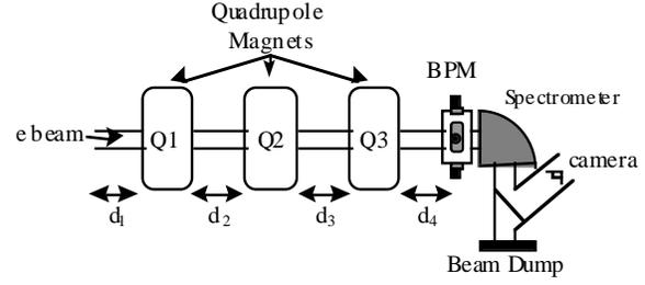
Figure 4: Schematic of beam line section used for emittance measurements.
