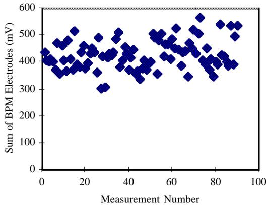
Figure 5: Sum of BPM Electrodes (beam intensity) versus measurement number for 90 beam shots.
