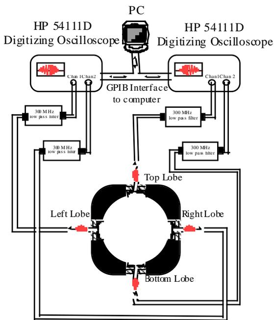
Figure 1: Schematic of data acquisition system.
