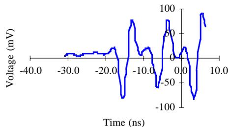
Figure 2: Typical voltage signal from a BPM electrode for two beam bunches.
