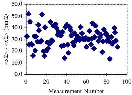
Figure 6:  $\langle x^2 \rangle - \langle y^2 \rangle$  (mm<sup>2</sup>) versus measurement number for 90 beam shots.
