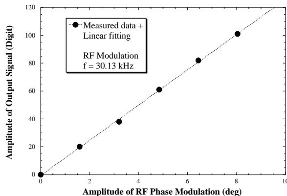
Figure 4: Calibration for converting the output digital data to the phase value
