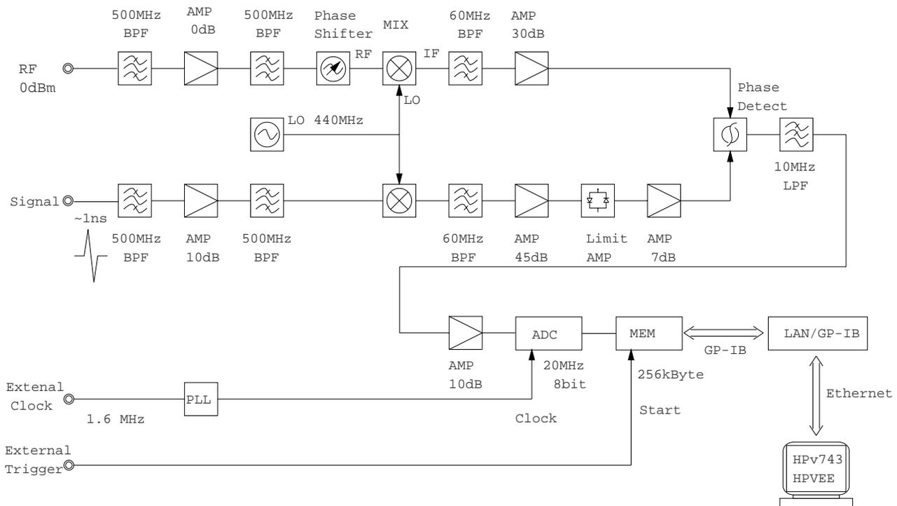
Figure 1: A block diagram of the phase detection circuit
