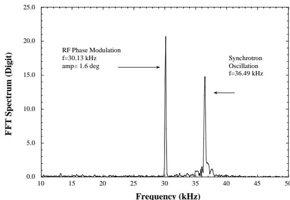
Figure 3: FFT spectrum of the data
