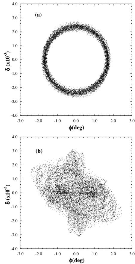
Figures 5: Longitudinal phase space plots of the oscillation caused by the RF phase modulation (a) and the single-bunch instability (b).
