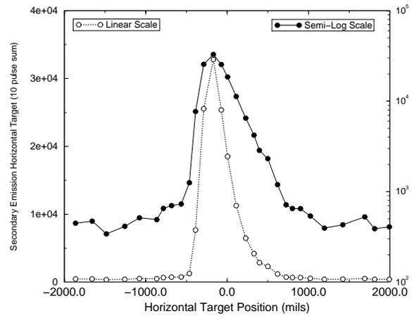
Figure 3: Secondary Emission from target for Horiz. Scan
