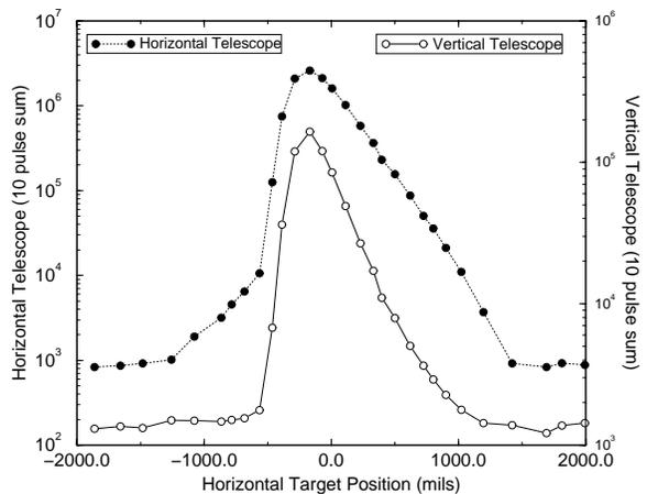
Figure 2: Horiz. and Vert. Telescope triples for Horiz. Scan
