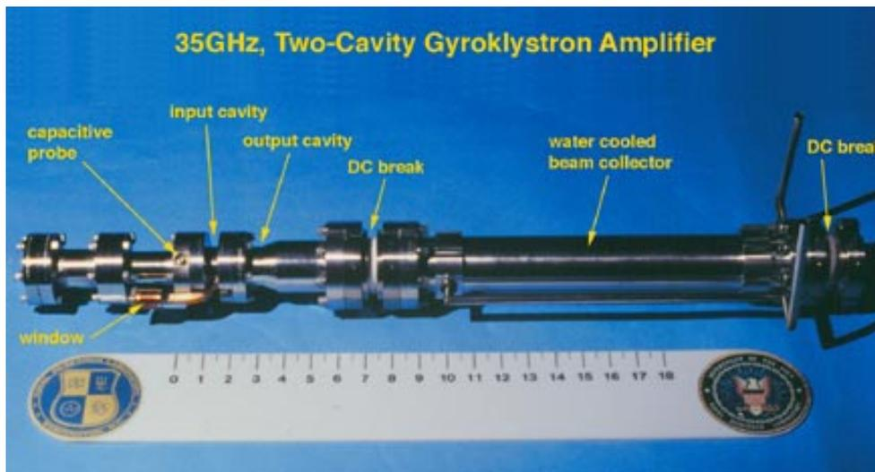
Figure 1. Two-cavity gyrokystron amplifier
