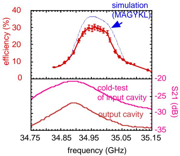
Figure 3. Large signal bandwidth
