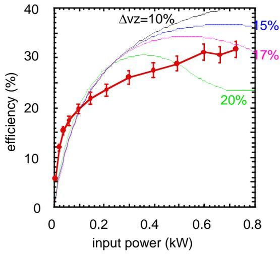
Figure 2. Experimental results on the drive curve. Simulation curves are  $\Delta v_z=10\%$ ,  $15\%$ ,  $17\%$ , and  $20\%$ .
