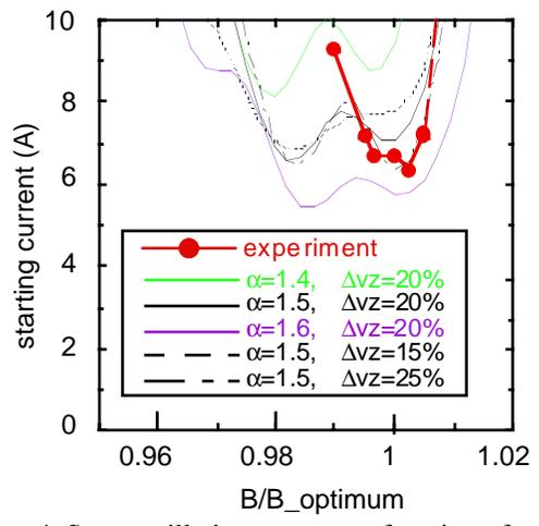
Figure 4. Start oscillation curve as a function of magnetic field detuning.
