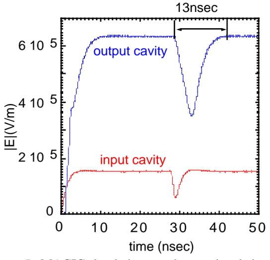
Figure 5. MAGIC simulations on the transient behavior of two-cavity gyrokystron. A phase shift by  $\pi$  in the input drive signal is switched on at 28nsec.
