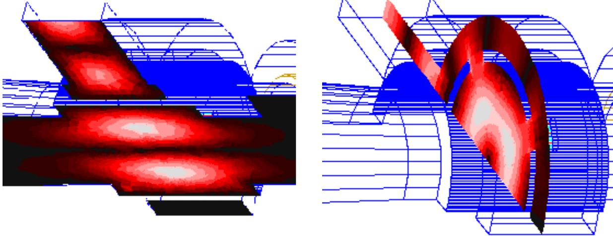
Figure 5. Intensity plot of  $|E|$  for transverse and axial cutplanes at 93.1 GHz.
