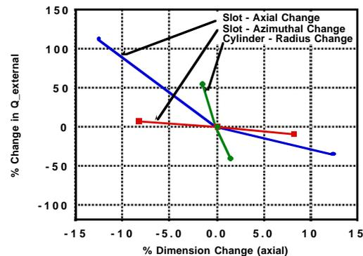
Figure 4:  $Q_{ext}$  change vs. dimensional change for a) slot axial size, b) slot azimuthal size, and c) cylinder radius.
