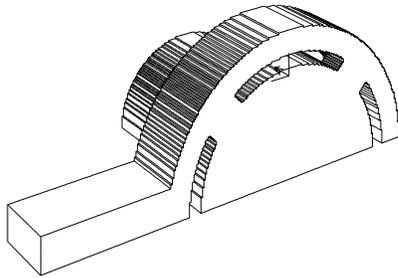
Figure 2: Input coupler simulation geometry for one quarter of the cavity.
