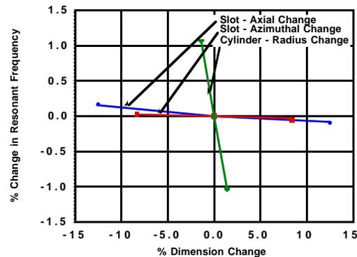
Figure 3: Resonant frequency change vs. dimensional change for a) slot axial size, b) slot azimuthal size, and c) cylinder radius.
