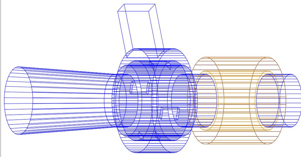
Figure 1: Schematic of input coupler geometry, including gun taper and drift tube dielectric. Vacuum/dielectric regions are shown.
