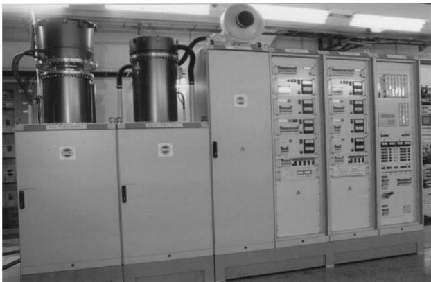
fig.1 One of the 400 kW amplifiers installed at CERN
