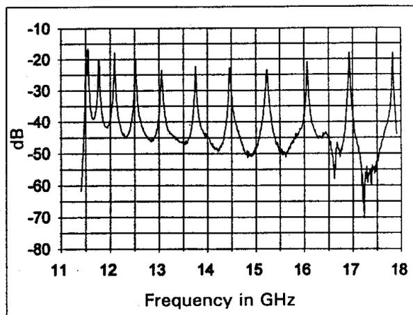
Figure 4 TM Modes frequency Spectrum of a Barbell Cavity as Measured with a HP8510C Network Analyzer
