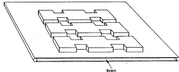
Figure 2 Schematic of a Planar Tugboat Traveling-Wave Structure (3 cells illustrated)
