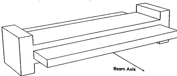
Figure 1 Schematic of a Planar Barbell Cavity
