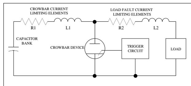
Figure 1: Simplified diagram of a typical crowbar circuit.
