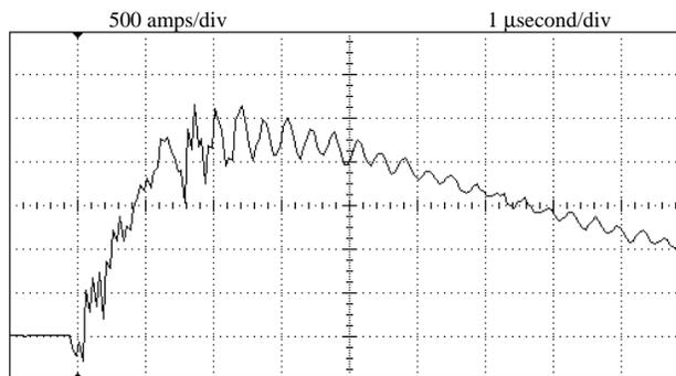
Figure 4: Current through the fault test wire.
