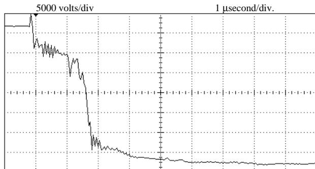
Figure 3: Ignitron voltage during fault.
