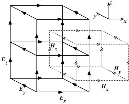
Figure 1: Yee cell structure of 3D discretisation
