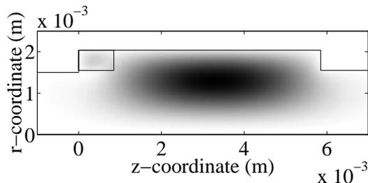
Figure 2: Gyroklystron cavity mode at 93.37GHz
