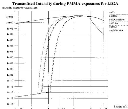
Figure 3: Transmitted x-ray intensity during PMMA exposures for DXRL at APS, energy (eV) vs. intensity ( $\text{W}/\text{cm}^3$ ).
