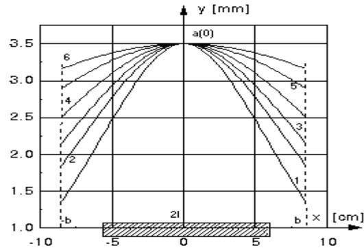
Figure 1. The shapes of the channel upper electrodes for different beam energies  $W$ : 1-50 keV, 2-100 keV, 3-150 keV, 4-250 keV, 5-500 keV, 6-1MeV ( $k_y/k_x=23$ ,  $\omega=1.256 \cdot 10^9$  1/s).
